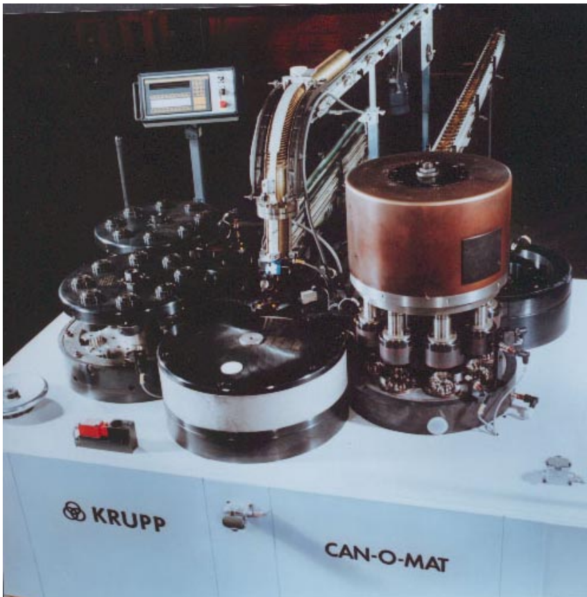
Figure 21 Seaming can ends
