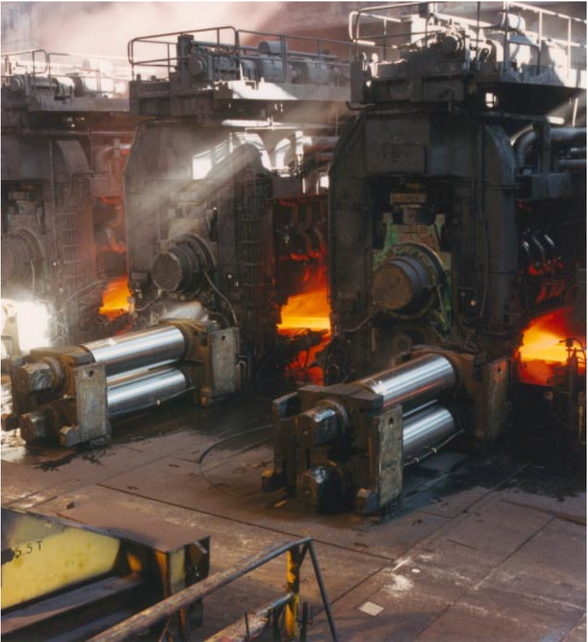
Figure 4 Typical hot strip finishing train
