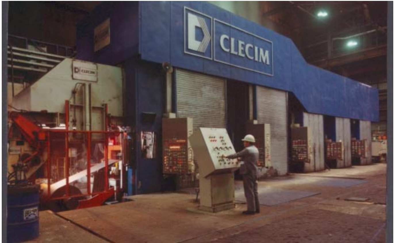
Figure 5 General view of five-stand tandem mill.
